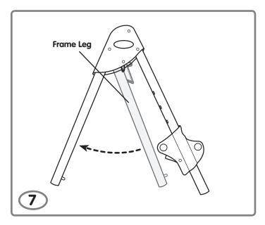
• Pull the frame leg out on each frame to open. Make sure it "clicks" into place.
